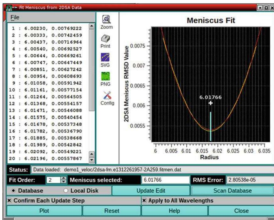
**Fig. 8.3** US3 dialog for the meniscus fitter. RMSD values from 2DSA Model files are plotted against meniscus position to identify the optimal meniscus position at the lowest RMSD
