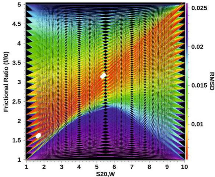
**Fig. 8.11** PCSA error surface heat map for SV data from a mixture of lysozyme and a 208 bp DNA fragment using a straight line parametrization. The white dots show the solutes found for the line that best fits the SV data. The color gradient indicates the RMSD value for each line
